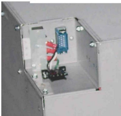
Mounted in rear: Signal and power input Connectors
