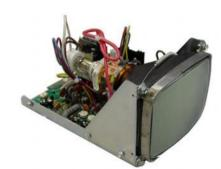
This Omni Vision monitor is offered in an open frame chassis or as a kit version product for applications where a small display is required and the input signal can be composite video or TTL or analog video with TTL sync. This low power CRT module is a great solution. The 5" CRT provides great viewing angles and higher brightness levels. The main circuit board is made of industrial grade epoxy/fiber glass reinforced material with an FR4 rating.
