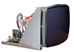
This Omni Vision monitor is offered in an open frame chassis or as a kit version product for applications where a small display is required and the input signal can be composite video or TTL or analog video with TTL sync. This low power CRT module is a great solution. This 12" CRT provides great viewing angles and higher brightness levels. The main circuit board is made of industrial grade epoxy/fiber glass reinforced material with an FR4 rating.
