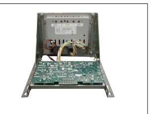
Kit version would include LCD module plus PCB for 10-pin card edge connection
