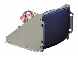
This Omni Vision monitor is offered in an open frame chassis for direct replacement of CRT display module in Dynapath equipment. In these chassis models the CRT and the deflection and signal processing circuit board are mounted in an open frame chassis assembly ready to be mounted in place. Omni Vision's main circuit board is made of an industrial grade epoxy/fiber glass reinforced material with an FR4 rating.
