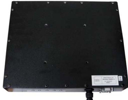
Picture is of special unit with single VESA mount pattern.
