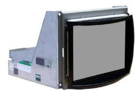
This Omni Vision 12.1" industrial LCD monitor is a direct drop-in for the Omni Vision model E144C-22 series industrial 14" color, open-frame CRT monitor open frame, assembled in sturdy metal chassis. It is designed to replace the 14" color CRT and it's associated electronics while maintaining high-resolution image requirements of wide-angle viewing and bright light output. This monitor operates as a standard plug-n-play VGA/XVGA monitor in an industrial environment.
